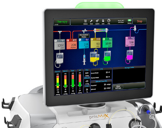
Fig. 2. The running mode screen on PrismaMax. Numerical data is mixed with a visual overview of the treatment status, for instance, the content status of the bags. Smooth colouring makes the view clear and systematic. ICU staff might not handle the machine every day and therefore, emphasis has been made to create a self-explanatory interface.
